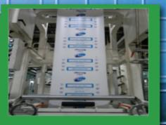
FFS Rolls are developed for different FFS (form-fill-seal) machines.
